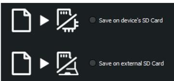
Save scenes to a micro SD card (Class 10) installed in the device's SD card reader or in the computer drive. The card must be CLASS 10, formatted in FAT or FAT 32 with a maximum capacity of 256 GB. It is recommended to use the largest allocation unit size available when formatting.
