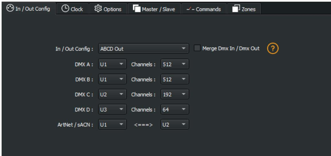
Assign any universe of the software to any DMX line assigned to output, choosing line by line (U1, U2...).
