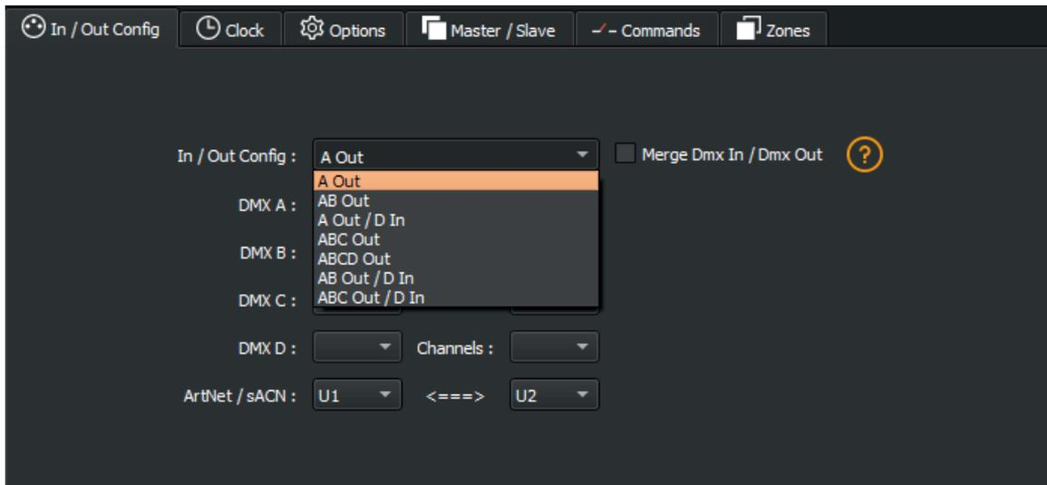
Available configurations will be displayed depending on the connected device depending on whether it has 1.2 or 4 DMX lines.
