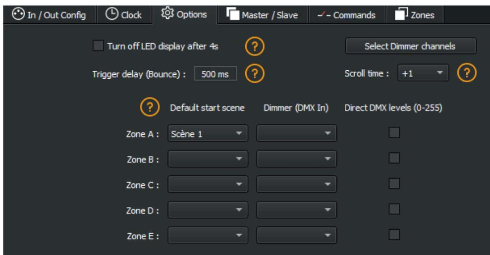
For devices with an LED display, turn it off after 4 seconds of inactivity by checking the option.
