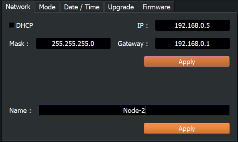
The screenshot shows the "Network" configuration tab in the DeviceTool interface. The "DHCP" checkbox is checked, indicating the device is in DHCP mode. The "IP" field is set to 192.168.0.5, the "Mask" is 255.255.255.0, and the "Gateway" is 192.168.0.1. An "Apply" button is visible below these fields. The "Name" field is set to "Node-2", with another "Apply" button below it. The interface includes tabs for "Network", "Mode", "Date / Time", "Upgrade", and "Firmware".
