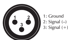
DMX-input XLR mounting-plug:
