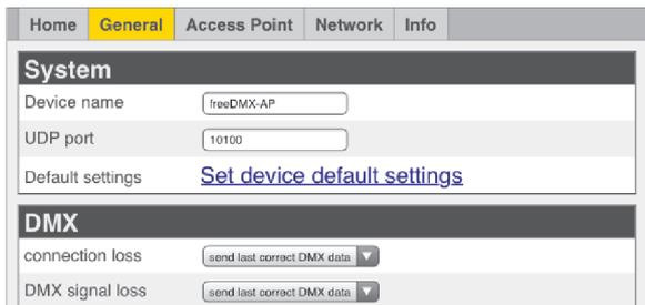
The screenshot shows a web interface for configuring a freeDMX AP. At the top, there are navigation tabs: Home, General (selected), Access Point, Network, and Info. Below the tabs, there are two main sections: System and DMX. The System section includes fields for Device name (freeDMX-AP), UDP port (10100), and a link for Default settings (Set device default settings). The DMX section includes dropdown menus for connection loss and DMX signal loss, both set to send last correct DMX data.
