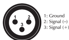
DMX-input XLR mounting-plug:
