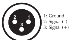
DMX-output XLR mounting-socket:
