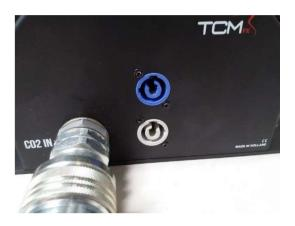
The Turbo Jet has a Powercon In and a Powercon Out connection.
