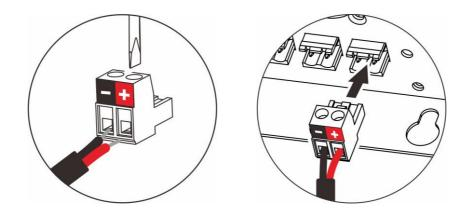
DarkFX Spot 510 IP is wired to output terminal of DarkFX Drive 4. Each output terminal can connect one DarkFX Spot 510 IP fixture.
